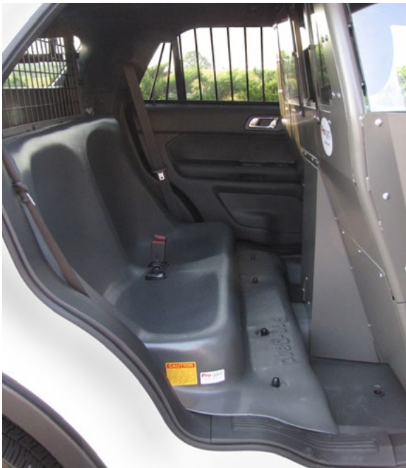
Transport Seats and Floor Pan shown in the Ford Police Utility Interceptor
